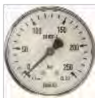
Fig. 3 Pressure gauge with scale for inlet pressure
