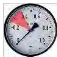
Fig. 5 Pressure gauge with scale for the dispensing (operating) pressure (0.25-0.4 bar)
