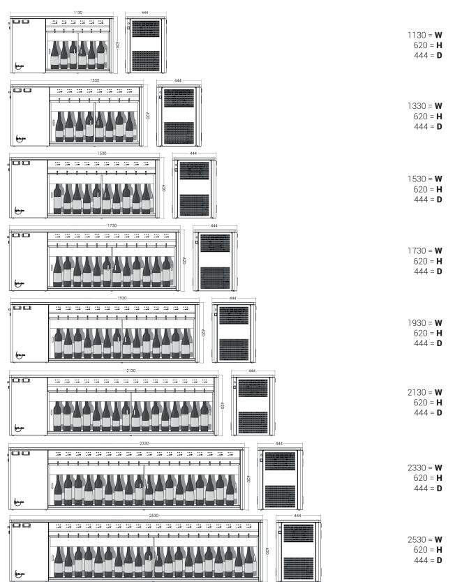
Note: For optimal efficiency and flawless operation foresee a min. 10cm of well-ventilated space to the side of cooling engine compartment. Split engine dispensers don't require free space. The in/outlets for power, inert gas and condense water can be guided through the side or through the bottom plate of the engine compartment.
