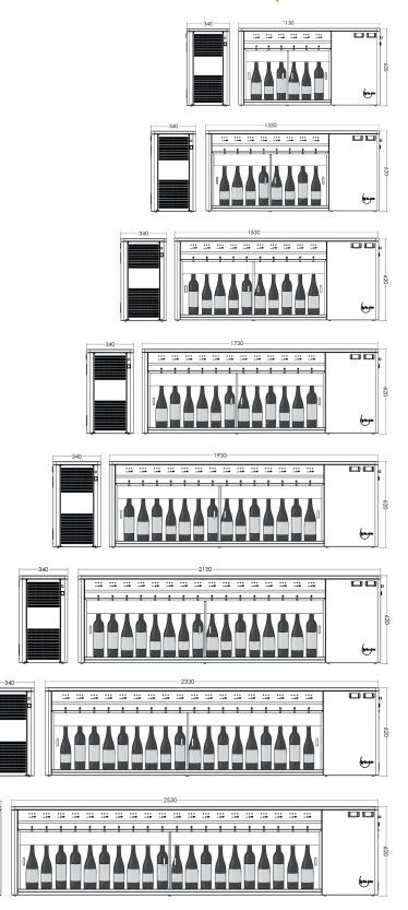
Note: For optimal efficiency and flawless operation foresee a min. 10cm of well-ventilated space on the side or behind the cooling engine compartment. The cooling engine compartment can be mounted either on the left or right side of the dispenser. Split engine dispensers don't require free space. The in/outlets for power, inert gas and condense water can be located at the back, on the side or through the bottom plate of the engine compartment.
